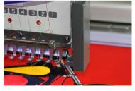
Camera positioning device Aids in correcting position and direction of designs in the case of improperly hooped items to ensure a precise embroidery outcome.
