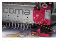
Cording device Easily create an embroidery effect with the cording device, which lays cord on fabric and attaches the cord with transparent zigzag stitches.
