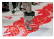
Boring device This device punctures holes into embroidered designs and encloses the raw edges with stitches to create a beautiful effect within minutes.
