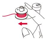
9. Once the spool is full, it rotates slowly. Release the pedal or stop. Push the bobbin winder spindle to left.
