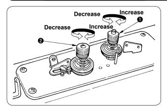
Tension post No.1 • is used to adjust the thread tension to sew on the button and a relatively low tension will be enough.
