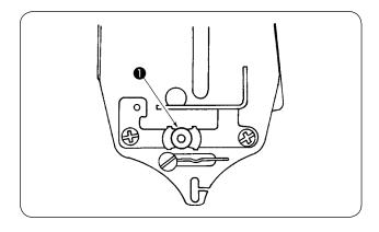
When the machine fails to form a seam at the start of sewing and starts to form it after it has run a while, adjust the thread tension guide on the face plate if the aforementioned trouble cannot be corrected by adjusting the thread pull-off lever.
