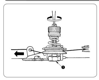
Turn the hand pulley as you draw the thread in the direction of the arrow as illustrated and you will find a point at which the tension disk on tension post No.2 releases the thread. At this moment, the standard distance from the top end of the needle bar bushing (upper) to the top end of the needle bar is 54 to 56 mm. Perform the following adjustments especially when the undermentioned troubles occur frequently.
