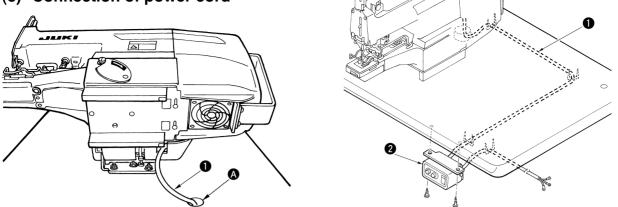
1) Tilt the sewing machine and put out cord ① coming out from the sewing machine to the lower side from hole ② in the table.
