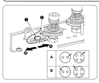
Adjustment of thread hauling amount is performed by loosening setscrew **1** and move the position of thread guide **2**.
