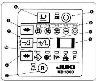
In the state that  $\pm 1/-$  switches **2** are simultaneously pressed, turn ON the power, and the memory switches are in the state of setting.
