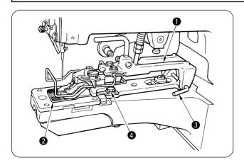
In order to install the attachmenton the machine, you may have to remove the button clamp mechanism 1 or feed plate 2. Dislocate a snap ring from button clamp installing stud 3, and you will be able to remove button clamp mechanism assembly 1. Remove setscrews 4, and you can remove feed plate 2.
