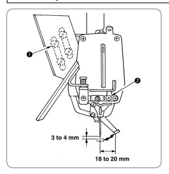
The standard thread catching point at the top end of the wiper should be 3 to 4 mm away from the tip of the needle and 18 to 20 mm away from the center of the needle at the stop position of the sewing end.
