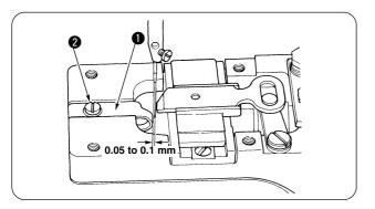
Loosen screw 2 and provide a 0.05 to 0.1 mm clearance between the needle and needle guide 1 by moving needle guide 1 to the left or the right when the needle bar is in the lowest position of its stroke.
