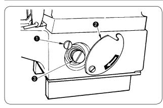
Slightly loosen knob ① located on the right side of the sewing machine, turn cover ② in the direction of the arrow, and you will find hand pulley ③ inside it. The rotating direction of this pulley is in the direction of the arrow.
