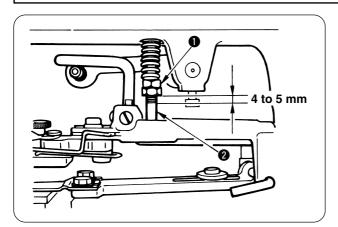
The standard work pressing force is obtained by turning nuts **1** and providing a 4 to 5 mm clearance between the bottom face of two nuts **1** and the bottom end of the screw of pressure adjusting bar **2**.
