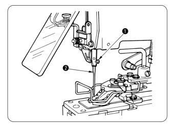
☆ The needle of TQx7 #16 is attached to the sewing machine.
