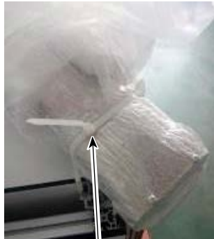
Cut the cable clip band to detach the sewing machine parts.
