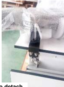
Cut the cable clip band to detach the sewing machine parts.
